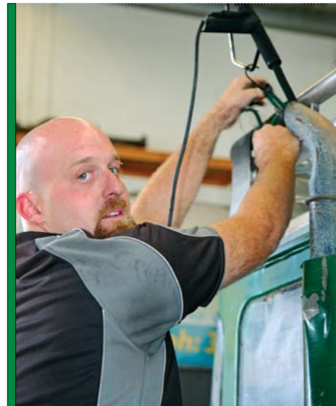
Steve O'Donnell spends his weeks working on fourbies and his weekends on the tracks himself! Here he's fitting an exhaust gas analyser, which allows the AMMS team to get the air-fuel ratio absolutely perfect. Milo gained power and economy!
