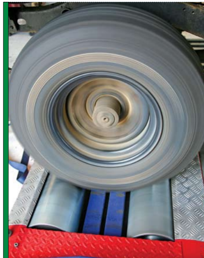
Wanting to know what would happen with a boost increase but the same fuel setting, I got the lads to give her another run. The result, as you can see from the graph, was a slight decrease in power to 74.2. Like Glen said in his best Roothy-tech talk, "diesels need more fuel to make more bang!"
