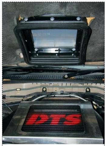
A rubber seal is fitted to the underside of the bonnet to push against the top of the intercooler heat shield
