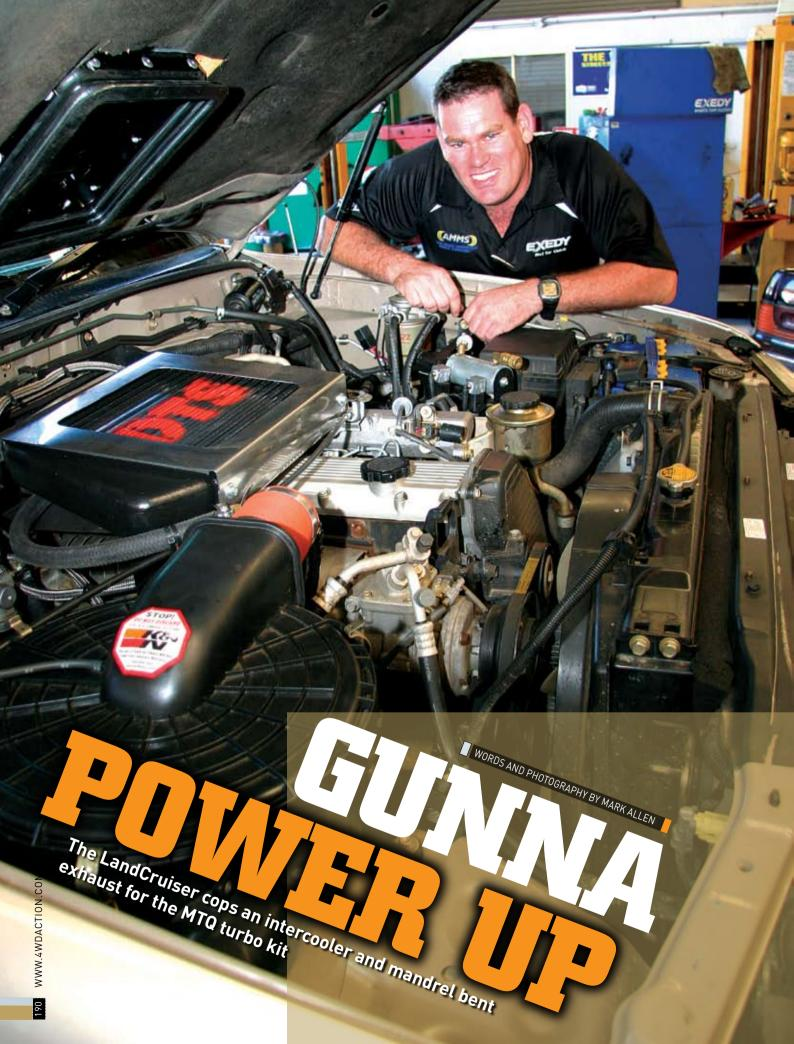
ast issue. AMMS in Brisbane installed the brilliant MTQ turbo kit that consists of a DTS water-cooled Mitsubishi TD05H turbo and all associated fittings. I was keen to transform the big, lazy 100 into a decent long-distance hauler. regardless of steepness of terrain or type of trailer in tow, so fitting an intercooler was a sure-fire way to finish off the power upgrade.
